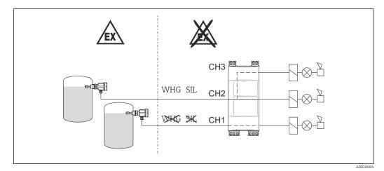
5. Channel CH2 is used for point level measurement with two level relays
